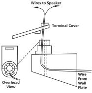
openings on top: a round screw hole, and an arc-shaped opening in front of it. The speaker cable should be threaded through the arc-shaped opening, not the screw hole.
